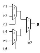
• Given the following inputs, provide the resulting function *g* (minimize the function).
